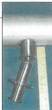
FIGURE 5. This low-profile device, a bubble-cap spray, can be used to clean overhead vapor lines that can not be flushed. It sprays upward and across to form a falling film that wets the sides of the riser and sweeps away soil
